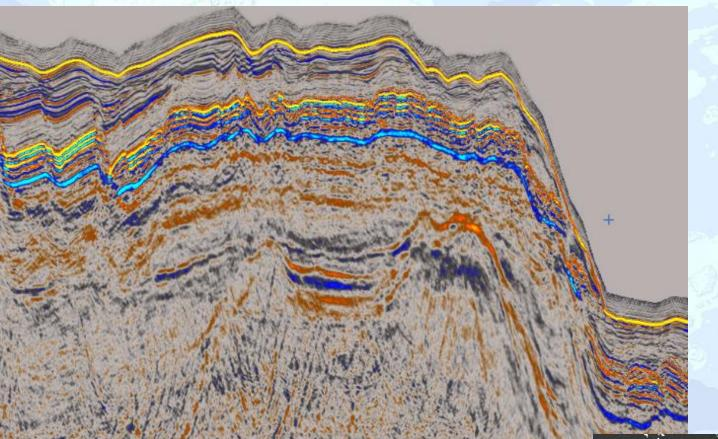
WD at structure: 430 m TWT of structure: 950 msec Structure width: ca. 7 km Reefal carbonates "atoll type", sealed by onlapping lagoonal seds. and Messinian Evaporites
