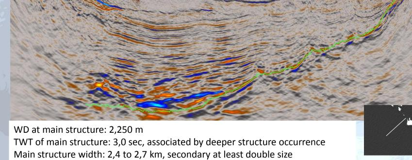
TWT Messinian Salt thickness: min. 100 msec (seal) Cretaceous carbonates erosional surface in green
