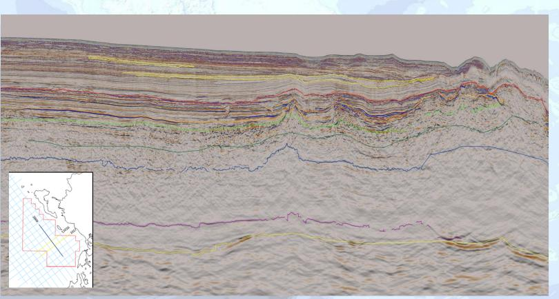
WD at structure: 1,590 m TWT of structure top: 2,9 sec Isolated carbonate build up sealed by Neogene pelagic seds. and Evaporites Max width: 9 km, 3 km each rim Various channels to be observed
